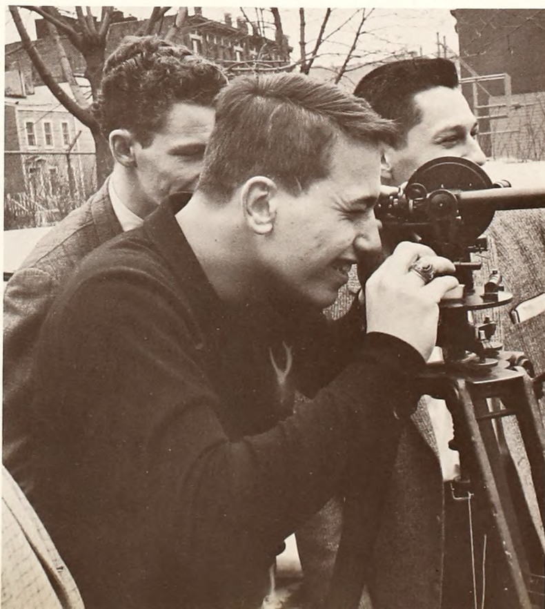
FRANK RUSSO-ALESSI applies trig theory to surveying transit in determining elevation angle of College building.
